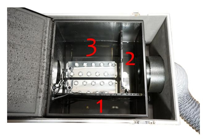
The Water Low FOG 3000, contains 3 different tanks. You can fill with water all of them, as they are connected. As the fog machine operates, the water level in tank 3 reduces. An electric pump then will
